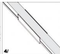
4/ Fix led strip completely into the fixed clip, led strip subplate must be parallel to the top edge of fixed clip
