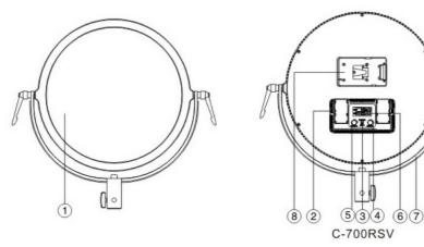
1 Front diffuser panel 2 Battery release button 3 DC input
